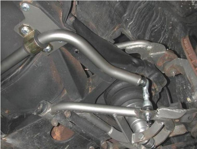
7. Apply lithium grease to the poly bushing. Install the bushing over the sway bar, and then place the bushing strap over the bushing.
