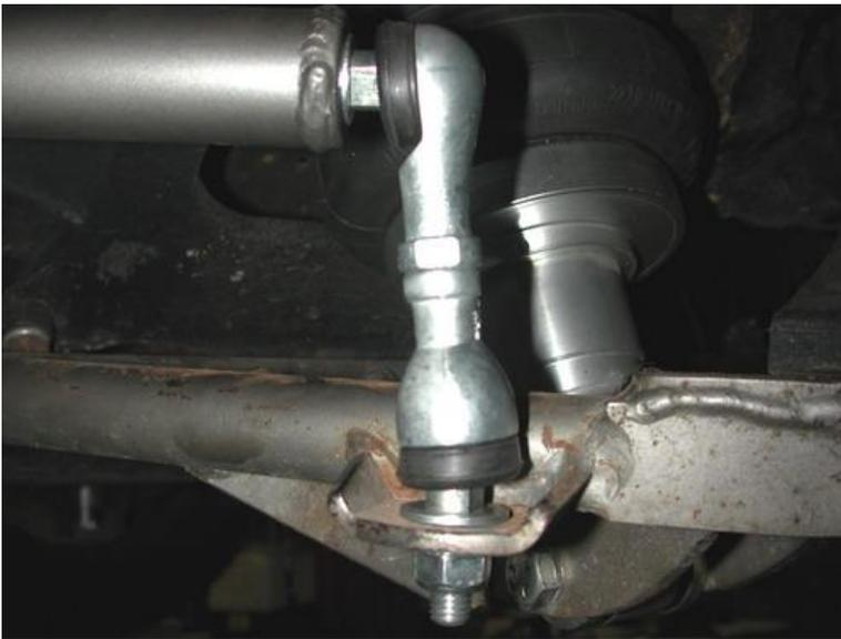
9. Bolt the 90 degree end of the PosiLink to the sway bar. A 3/8" flat washer and 12mm lock washer must be installed between the PosiLink and the bar.
