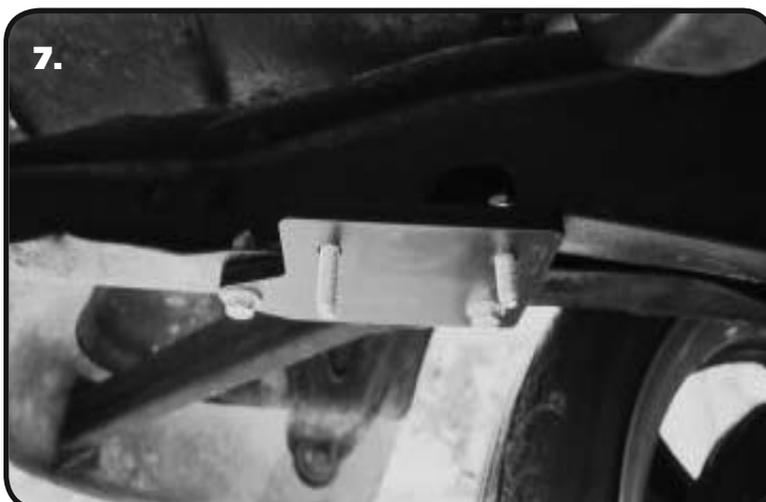
7. Install 3/8" Flatwashers on (2) 3/8" x 1 1/4" Hex bolts. Install them through the top side of the of the remaining holes in each Mounting Plate with the threads pointing down. The rear bolt will also go through the frame rail.
