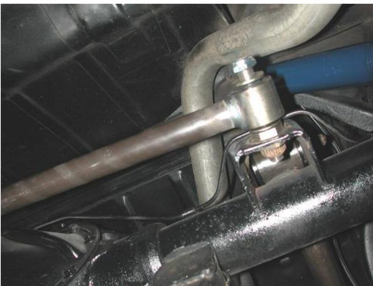
2. Replace the factory panhard bar with the new one using the new stud and hardware supplied. Insert the 5/8" Inside Diameter R-Joint Spacers into the R-joint of one end of the Panhard Bar.
