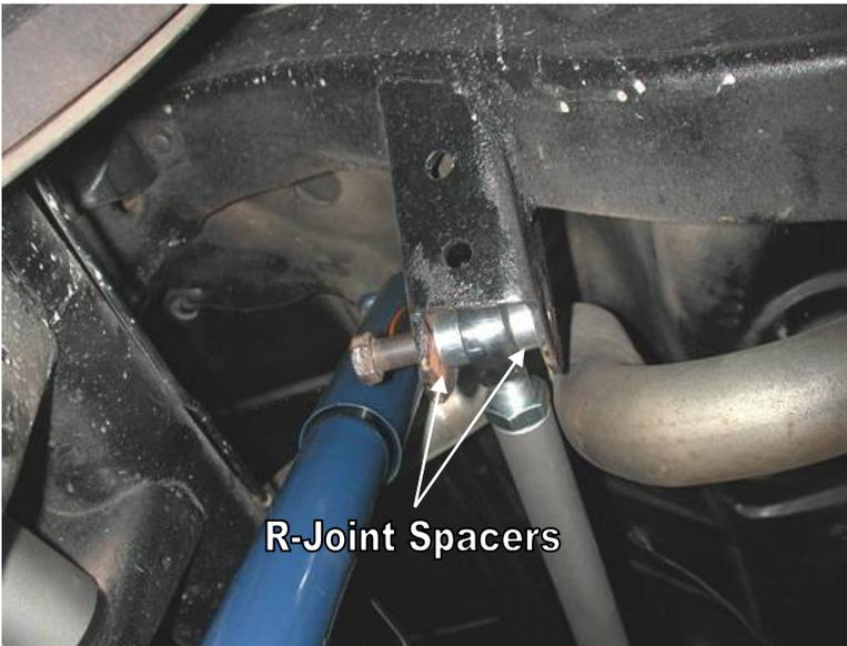
3. The other end of the Panhard Bar will attach to the frame using the 9/16" x 3" bolt and Nylok nut. Insert the 9/16" Inside Diameter R-Joint Spacers into the R-joint
