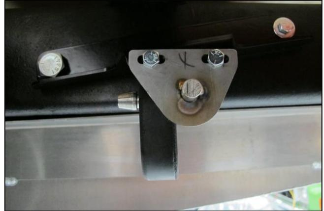
Driver's Side Dual Side Exit System Tailpipe Hanger Installation
