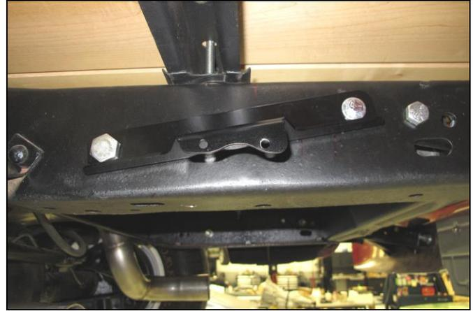
Driver's Side Tailpipe Hanger Frame Bracket Installation
