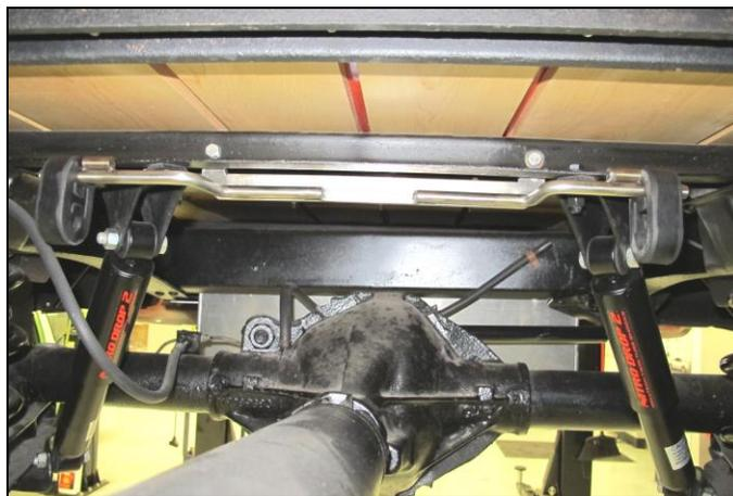
Front Tailpipe Hanger Frame Bracket Installation
