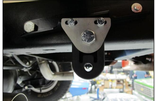
Driver's Side Dual Rear Exit System Tailpipe Hanger Installation
