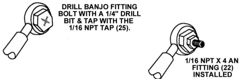
Figure 8 Schematic of "Drilled Out" Banjo Fitting
