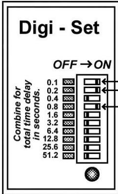
This time delay switch will allow you to activate a second stage of nitrous as a function of time.
