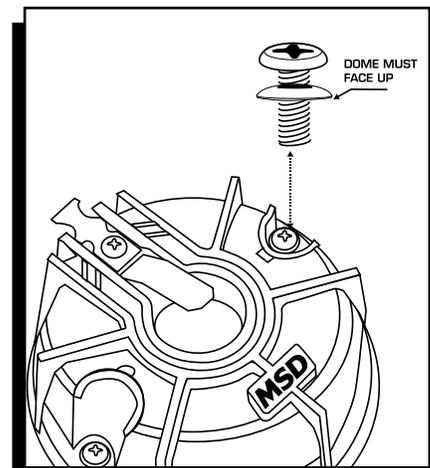
Figure 1 Washer Installation.
