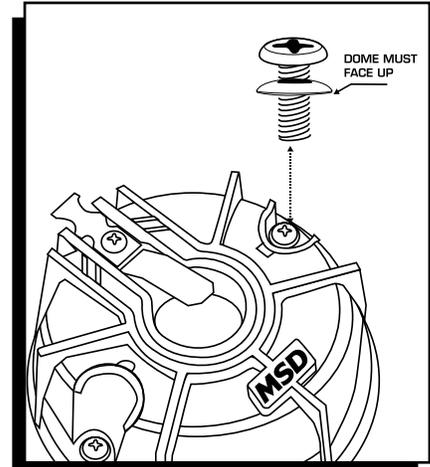
Figure 1 Washer Installation.
